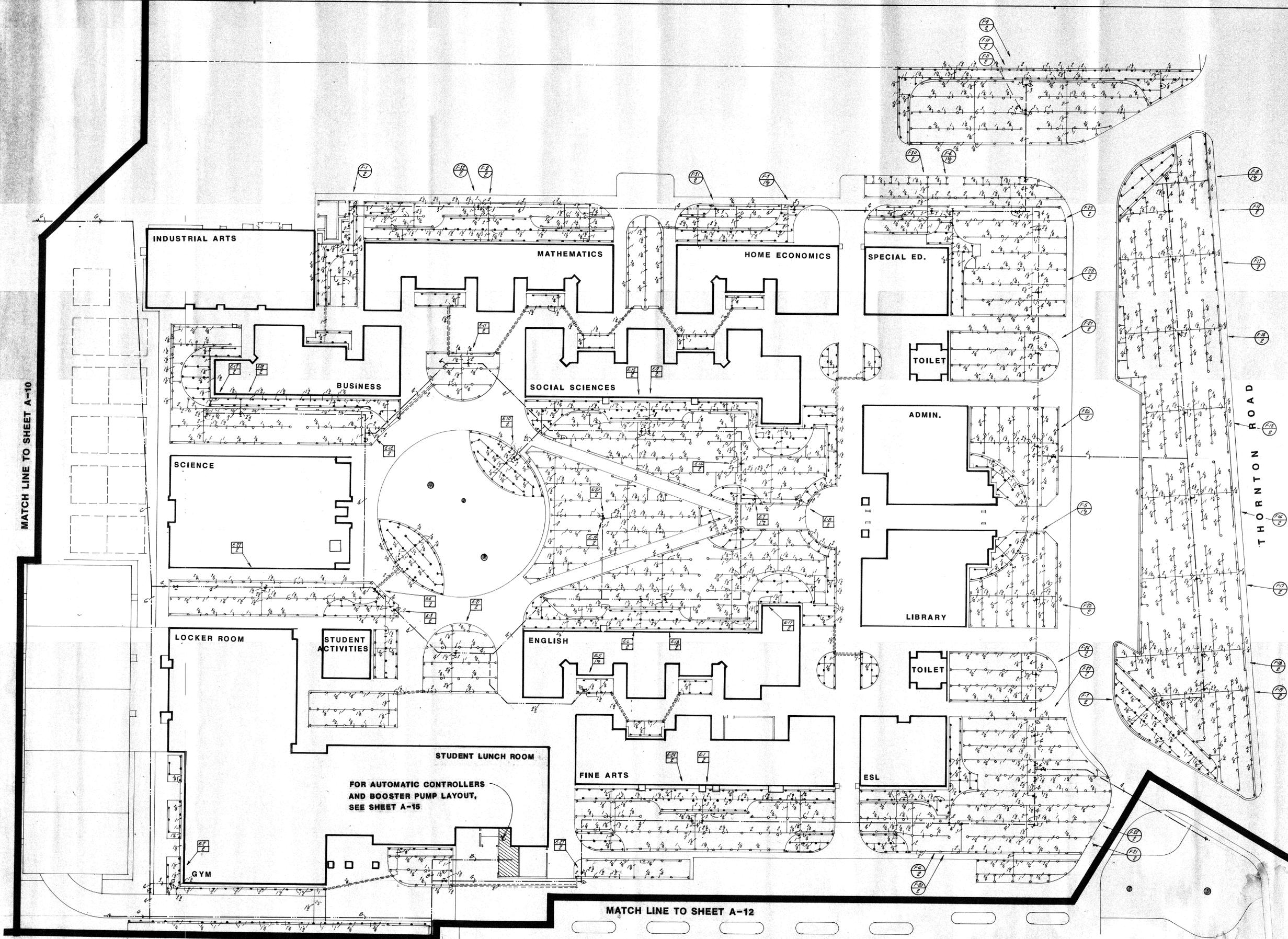
**BIDDERS NOTE:** THE PORTION OF SPRINKLER IRRIGATION SYSTEM TO BE DEDUCTED AND INCLUDED AS PART OF DEDUCTIVE ALTERNATE ITEM NO. 2 IS ALL THE LATERAL LINES AND SPRINKLER HEADS DOWN STREAM OF ALL AUTOMATIC CONTROL VALVES FROM "R" AND "P" CONTROLLER. MAIN LINE, AUTOMATIC CONTROL VALVES, GATE VALVES, QUICK CLOSURE VALVES, CONTROL WIRE AND AUTOMATIC CONTROLLER "R" AND "P" TO REMAIN A PART OF BASE BID.
