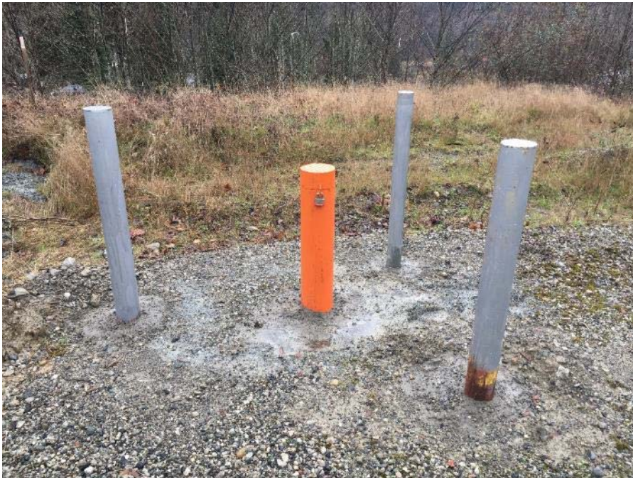
8. LOOKING EAST FROM THE NORTHEAST PORTION OF THE GRADED GRAVEL AREA AT ONE OF THE MONITORING WELLS OBSERVED ON THE SUBJECT PROPERTY. THE TOPOGRAPHY APPEARED TO STEEPLY SLOPE DOWN TO THE EAST BEYOND THE MONITORING WELL.
