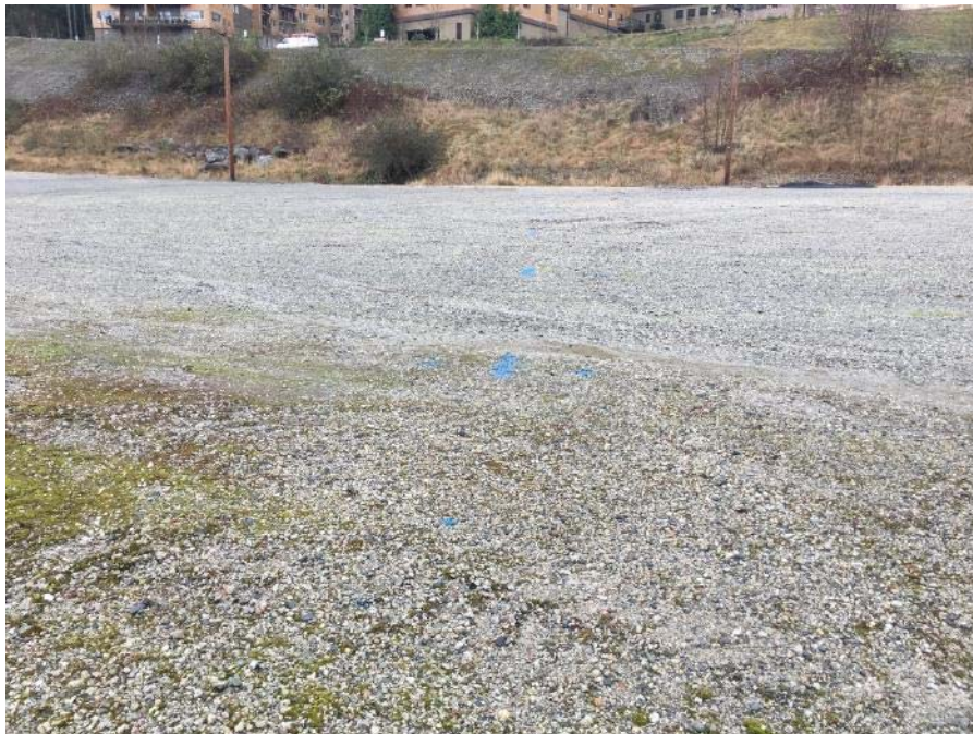
10. LOOKING WEST AT BLUE UTILITY MARKINGS ON THE GROUND INDICATING A WATER LINE BENEATH THE SUBJECT PROPERTY.
