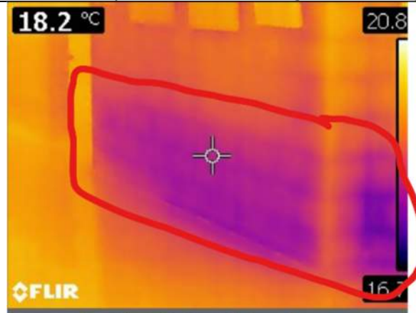
This corner near the ramp is where the water was actively observed entering the building.
