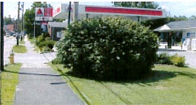
A mature shrubs next to a driveway could cause problems with visibility for cars exiting the driveway.
