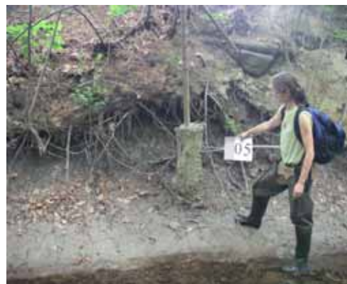
Hanging fencepost shows severe bank erosion near Station 1.
