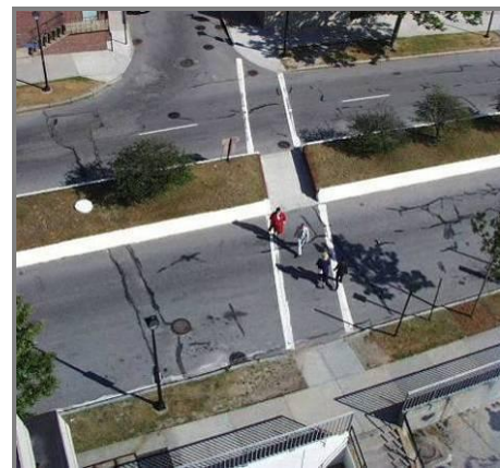
Median refuge islands break up a crossing and allow pedestrians to cross one side of a street at a time.
