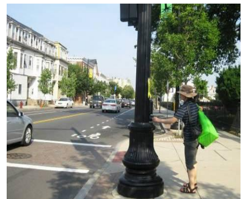
Pedestrian push buttons need to be very visible from the adjacent sidewalk.
