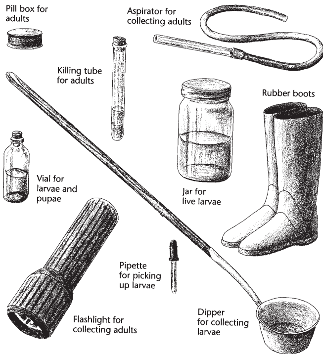
Fig. 3-6—Mosquito monitoring equipment. The most important device is a white enamel dipper equipped with a long handle for sampling larvae and pupae.
