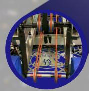
Photoeyes are used to evenly and reliably space apart Power Cells in the intake. Chain for durability, 8 wheels for shooting stability, and pneumatic wheels to increase traction and reliability during autonomous.
