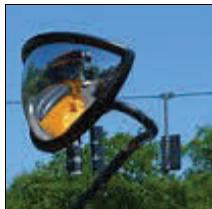
Learning the proper use of mirrors is vital to the safe operation of a school bus. Mirrors provide maximum visibility when they are free from defects, are properly adjusted and are kept clean. The adjustment of the crossover mirrors is still a major concern on many of the buses. Take time to use the mirror grids painted on the parking lots of the high schools throughout the county.
