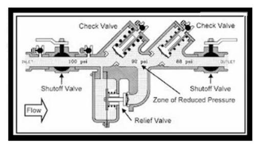
Backflow Preventers (also known as Reduced Pressure Devices) are essential in protecting the drinking water. They limit water traveling from your property back into the City's water system so that the system can provide clean, safe drinking water to you and all of our customers..
