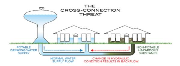
Backflow is the reversal of flow in a water system from the normal or intended direction of flow. Backflow prevention is necessary to prevent any potential contaminants or pollutants from entering the water distribution system from private plumbing systems; either from back pressure or back siphonage.
