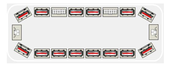
Peripheral Lighting: The following warning lights shall be installed in exact positions approved by NBEMS. All fixtures must be synchronized for proper Left to Right alternating of flash signals.
