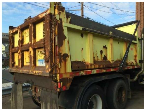
Picture shows the impact of salt on a Public Works dump truck used in Winter Storm Operations.
