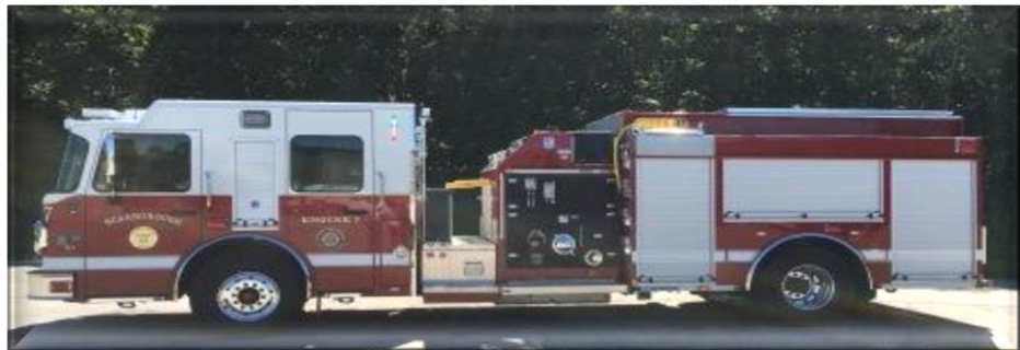
Smeal CAFS Pumper with 1,500 gpm pump & 1,000 gallon water tank
