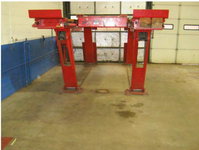
**Piston (center, under aboveground lift) with associated hydraulic controls against wall (left), automotive garage.**
