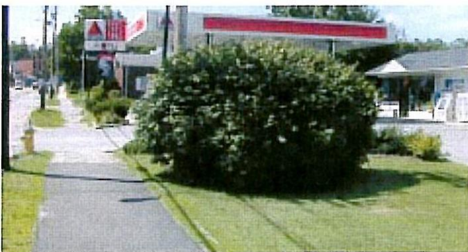
A mature shrub next to a driveway could cause problems with visibility for cars exiting the driveway.
