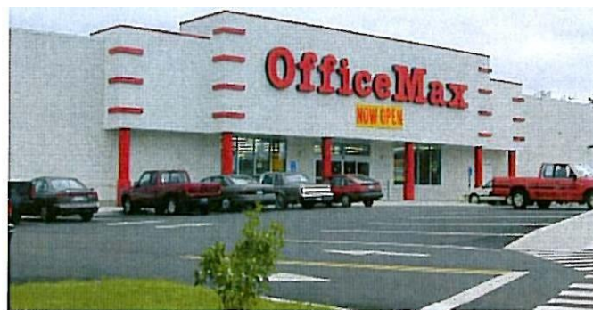
While the front plane of the wall of this building is broken, the offset does not collide to the ground. The projection becomes a billboard and the building is seen as a large box.
