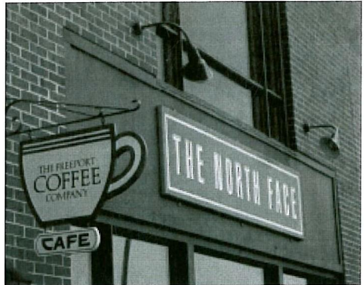
In both examples above and below the top-mounted light fixtures are well-located, aimed, and shielded so that only the sign is lit
