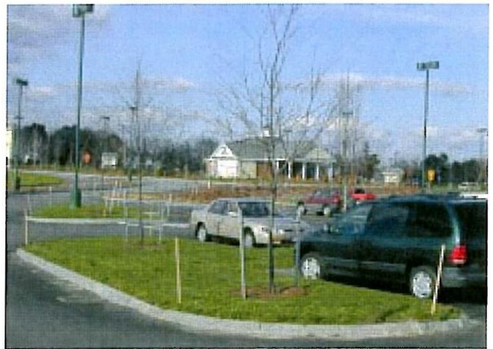
Wide parking lot islands provide ample room for tree growth and snow storage.
