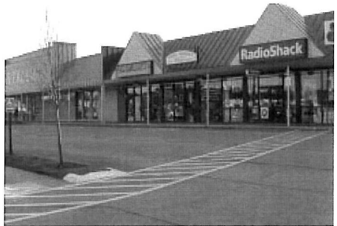
This circulation system results in excessive width in front of the storefronts and creates an auto-oriented environment. The painted walkway offers little contrast and leads to tire parking aisle.
