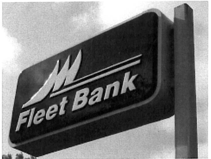
The sign's dark background and light lettering emphasize the bank's name while minimizing glare. Information occupies about 40% of the sign.
