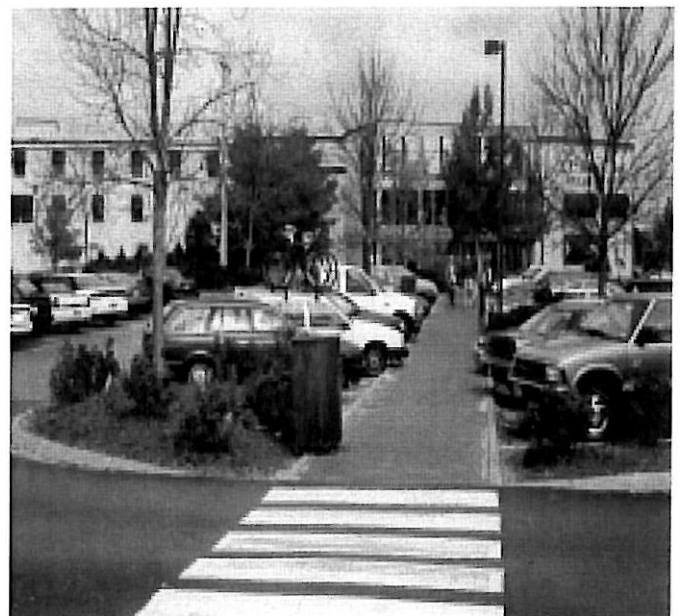
A wide walkway that provides a well-marked, attractive pathway to the main entrance. Separated walkways are more desirable than systems that end behind parked cars.
