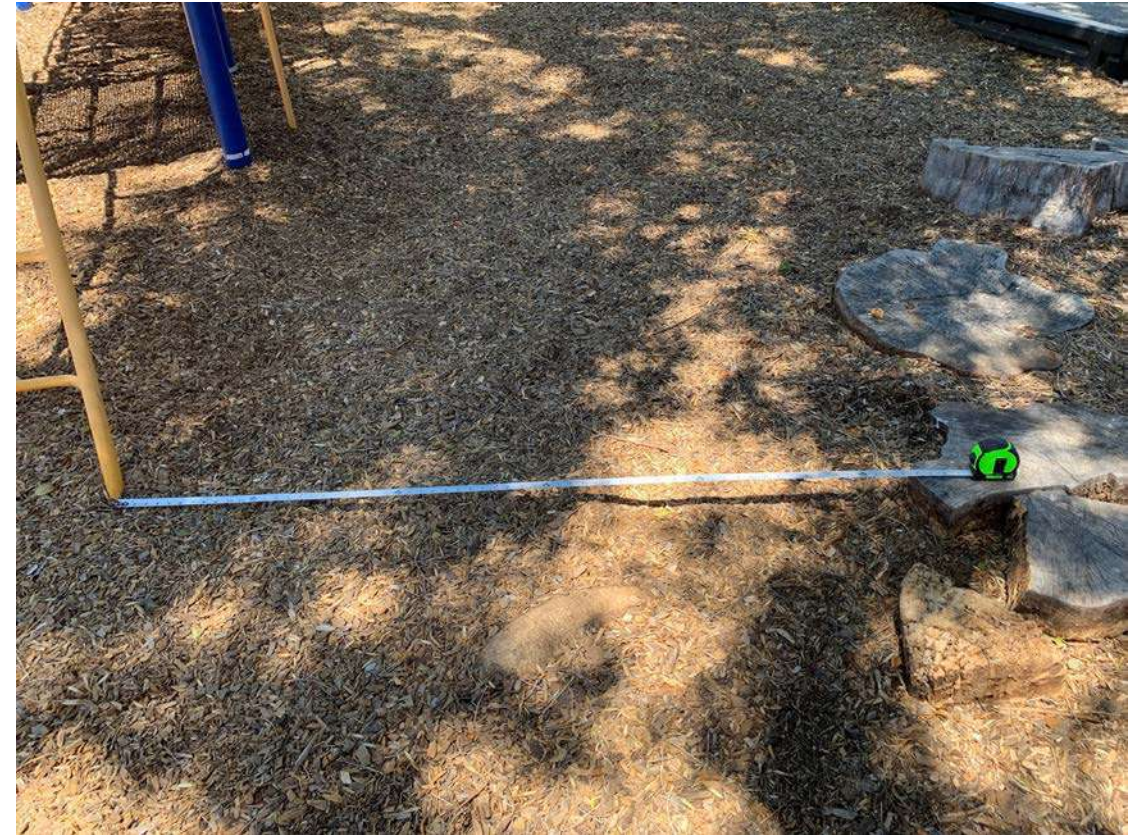
Use zone/Fall zone violation with Stumps.
