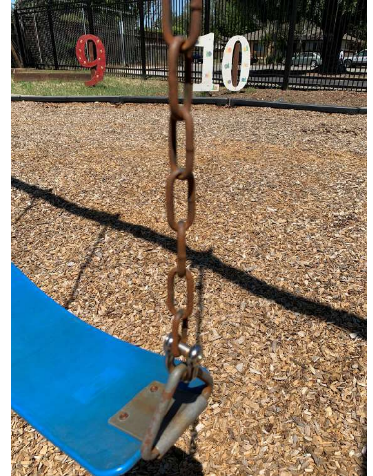
Corrosion on chains, seats, and fasteners.
