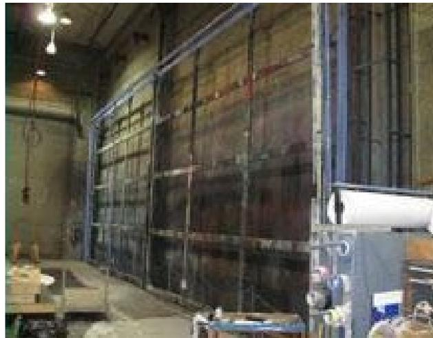
The ability to move the canvas up and down reduces the risk of falls by reducing the need to use ladders to access the upper reaches of the canvas. However, the floor opening in the floor through which the paint frame moves poses trip and fall hazards that could result in serious debilitating injuries or death.
