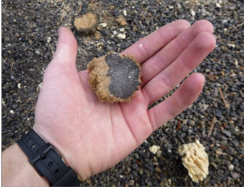
Figure D.3 Fiberboard cover board is dry.
