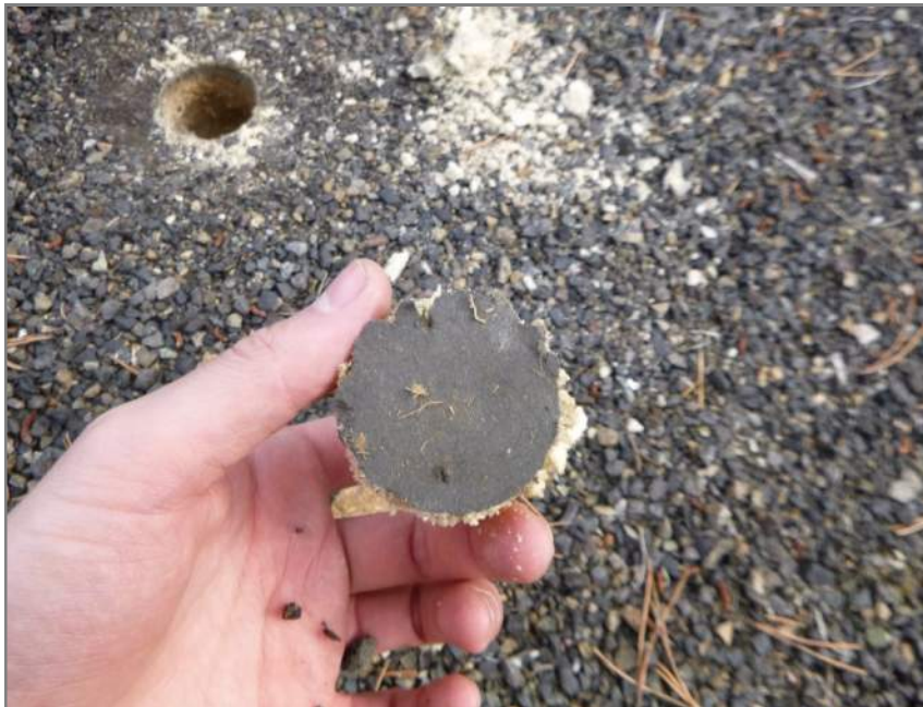
Figure D.10 Paper facer of insulation is intact and dry.
