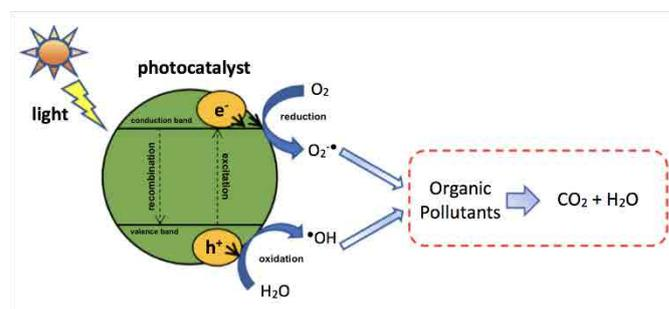
Fig.2 Visual Diagram of How a Photocatalyst Works (Source: nature.com)
