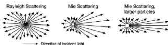
Fig.7 Visual Diagram of Mie and Rayleigh Scattering (Source: [14])
