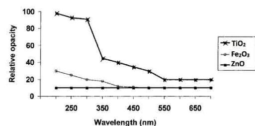
**Fig.6** Comparison of the Relative Opacities of Different Microfine Pigments (Source: [4])
