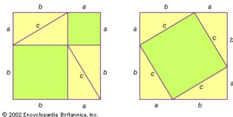
See how the yellow areas in the first diagram can be rearranged to form the second diagram and how this proves Pythagoras' Theorem.
