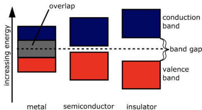
Fig.1 Visual Diagram of a Semiconductor and How it Differs from Metals and Insulators (Source: energyeducation.ca)
