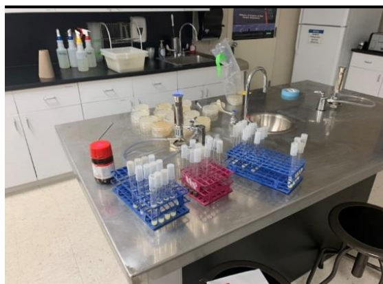
Figure 3: Serial dilutions of the spiked liquid MM broth from 10^{-1} to 10^{-6} . Additionally, the MM plates can be seen and the pyrene that was used to spike the plates. Photo credit: Sydney Smith.
