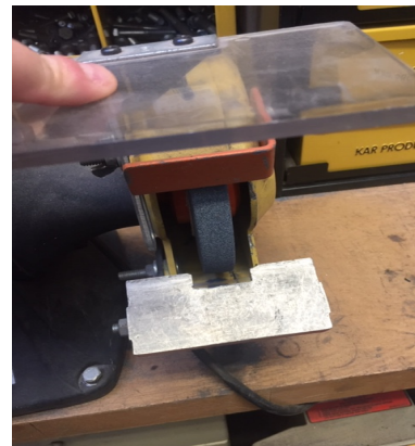
Bench grinder clearances need to be adjusted - corrected
