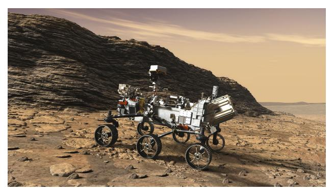
Perseverance is about the size of a car, it is 10 feet long, 9 feet wide, and 7 feet tall. It weighs 2,260 pounds which is less than the weight of a car. It landed in Jezero Crater which was a carefully
