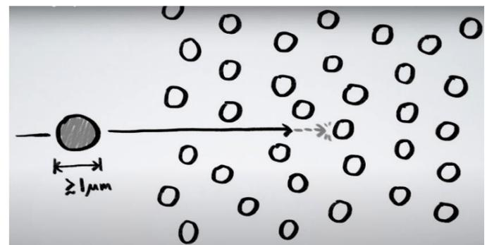
Figure 1: Capture by inertial impaction<sup>7</sup>
