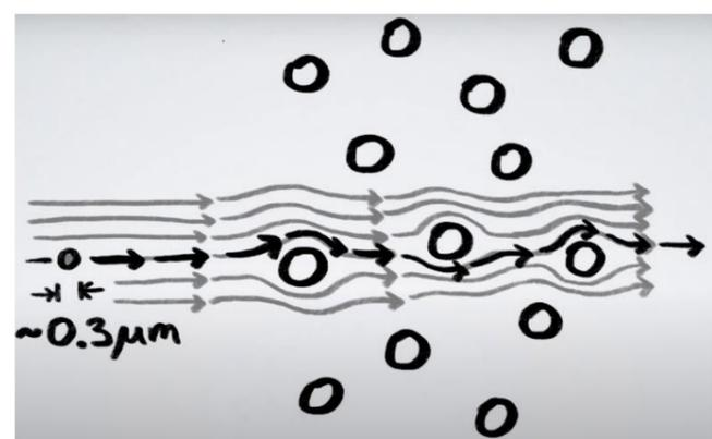
Figure 3: Motion of  $\approx 0.3\mu\text{m}$  particles around uncharged fibres
