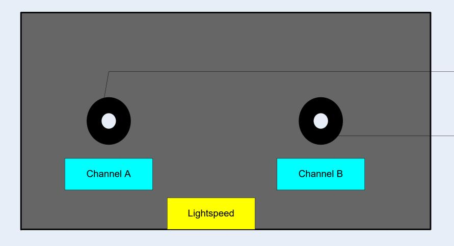
To return to Base settings Turn Channel A potentiometer all the way clockwise gently until it stops Turn Channel A counter clockwise until bottom of screw slot is pointing at 10 and 4 o'clock
