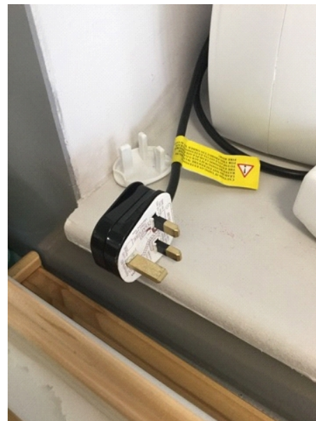
Fan heater plug in main pre prep classroom with card wiring label still attached even though unit was PAT tested.
