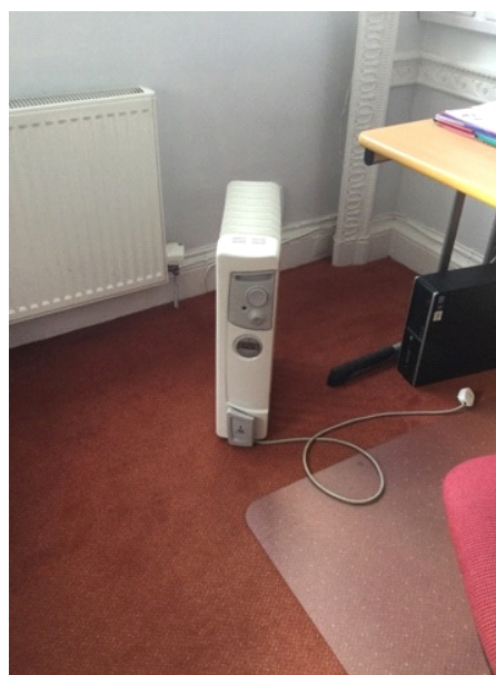
Oil filled radiator in first floor office leading from main stairwell missing feet.
