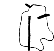
Fiber protrusion <5:1 Aspect Ratio
