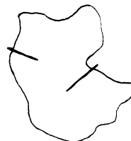
Fiber protrusion <0.5 micrometer
