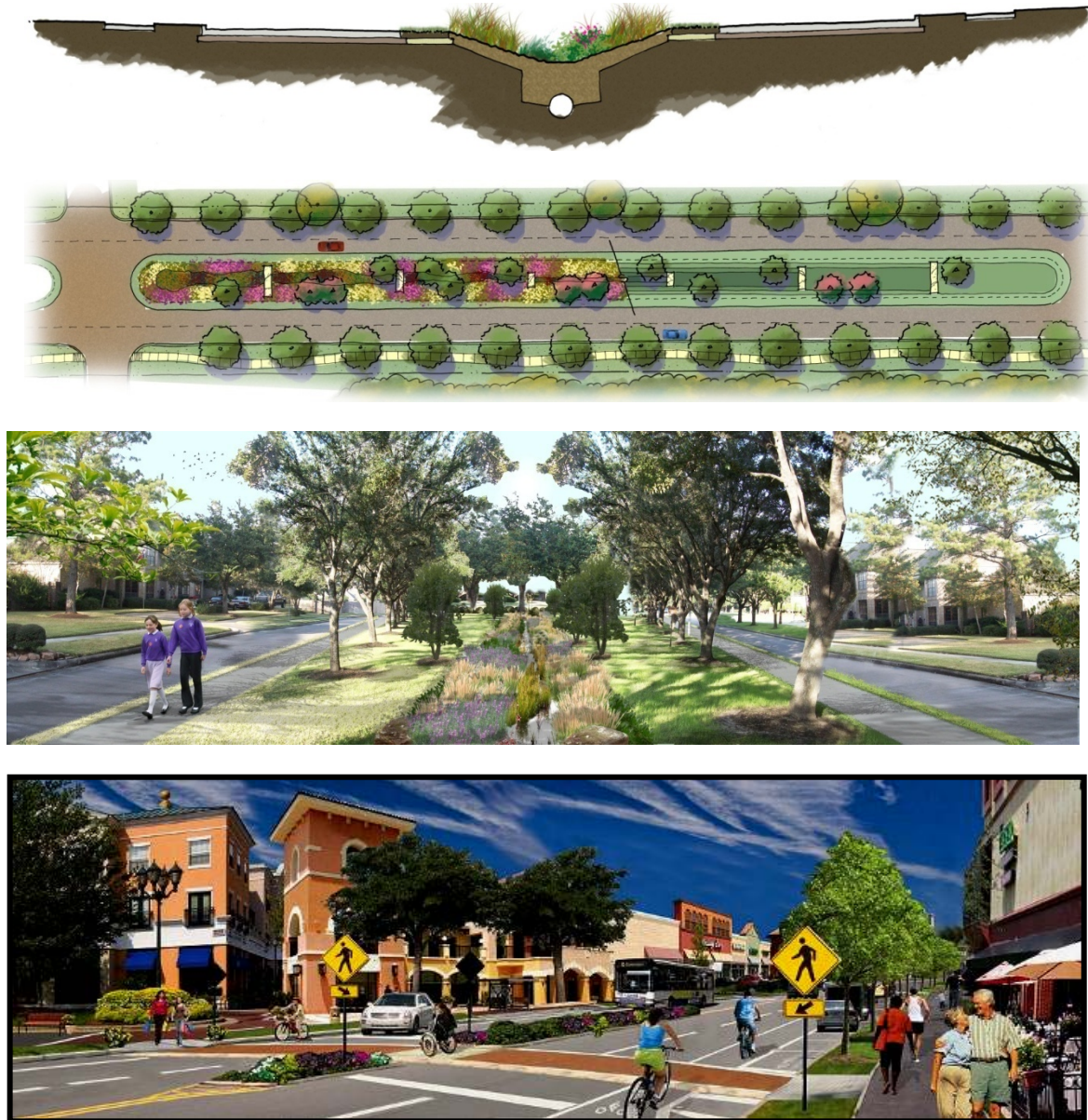
Figure 3.8 – Examples of center median infiltration/filtration systems
