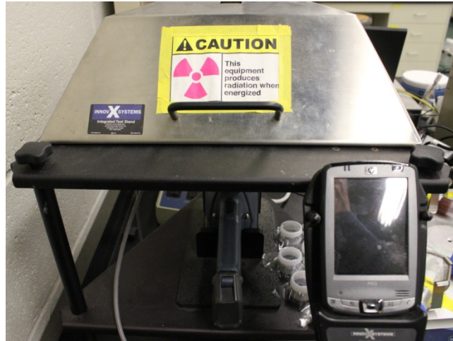
(b) INNOV-X Systems XRF analyzer
