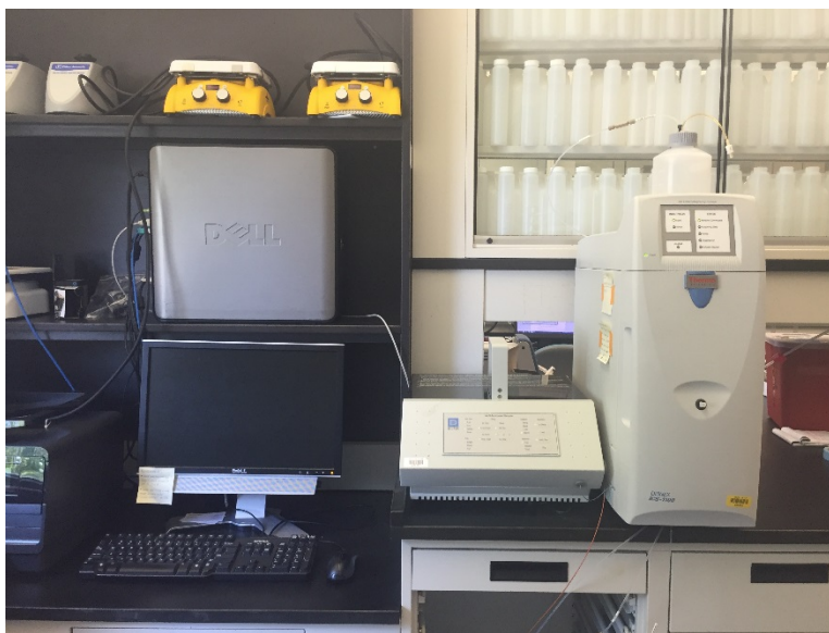
Fig. 5.7 DIONEX ICS-1100 ion chromatography
