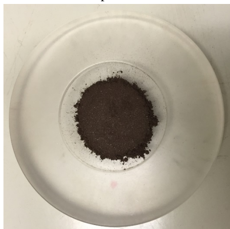
e) sample in the vehicle for XRD test
