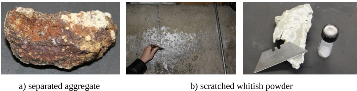
Fig. 6.1 Sample preparation for XRD testing
