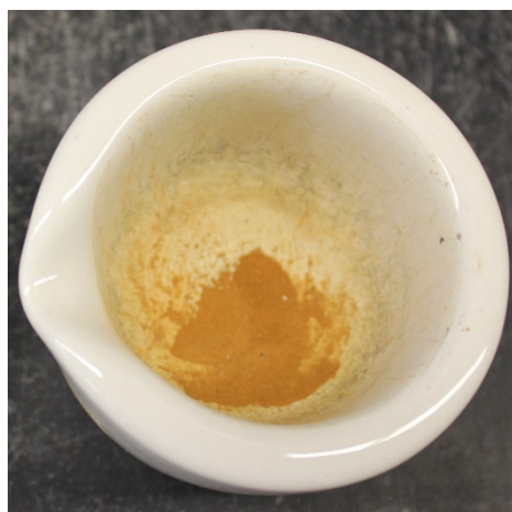
c) ground sample using mortar and pestle
