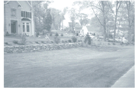
Figure 4.18 – Vegetative filter strip. Source: Connecticut, 2004.
