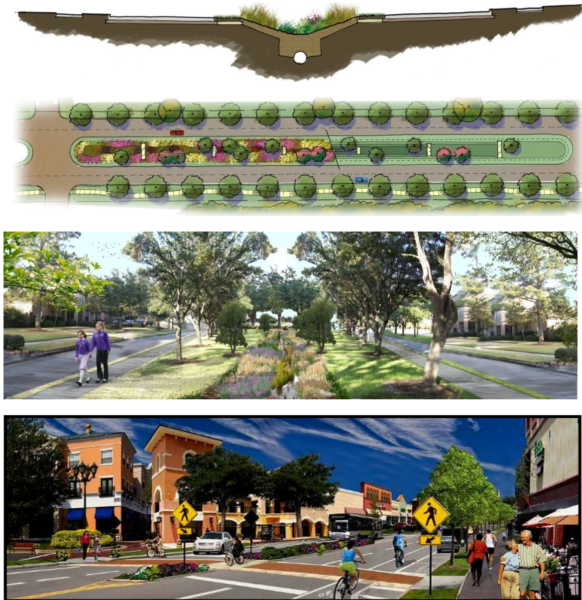
Figure 3.8 – Examples of center median infiltration/filtration systems
