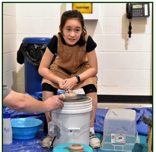
6th grader Grace demonstrates her working pottery wheel built from a ceiling fan motor.
