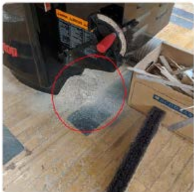
Accumulated combustible dust
