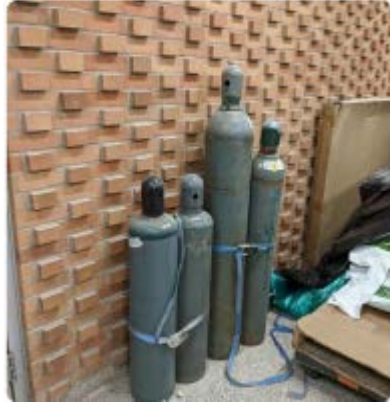
Cylinders not stored properly - Contractor
