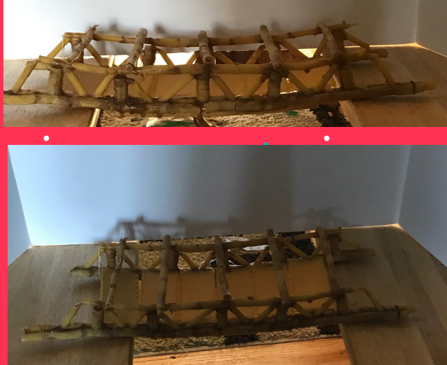
Caleb G.'s mixed Pratt/Howe Truss Bridge Design
