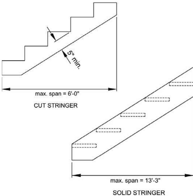
**Figure 29. Tread Connection Requirements.**
