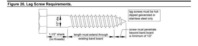
Lag screw installation requirements: Each lag screw shall have pilot holes drilled as follows: 1) Drill a  $\frac{1}{2}$ " diameter hole in the ledger board, 2) Drill a  $\frac{5}{16}$ " diameter hole into the band board of the house. DO NOT DRILL A  $\frac{1}{2}$ " DIAMETER HOLE INTO THE BAND JOIST.
