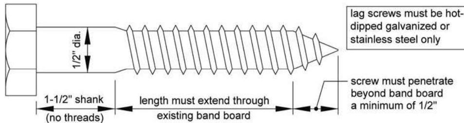
**Lag screw installation requirements:** Each lag screw shall have pilot holes drilled as follows: 1) Drill a 1/2" diameter hole in the ledger board, 2) Drill a 5/16" diameter hole into the band board of the house. **DO NOT DRILL A 1/2" DIAMETER HOLE INTO THE BAND JOIST.**
