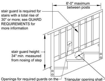
sides of stair treads shall not allow a sphere 4-3/8" to pass through. Triangular opening shall – not permit the passage of a 6" diameter sphere.
