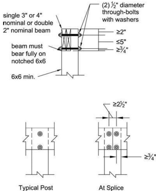
**Figure 8B. Alternate *Approved* Post-to-Beam Post Cap Attachment.**
