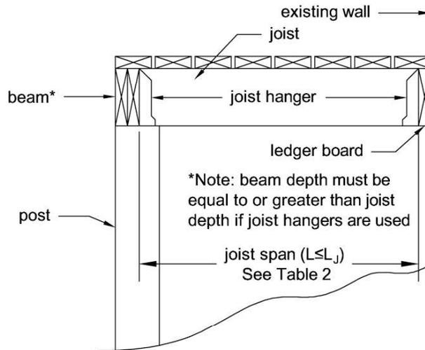
**Figure 2. Joist Span – Non-Ledger Deck.**
