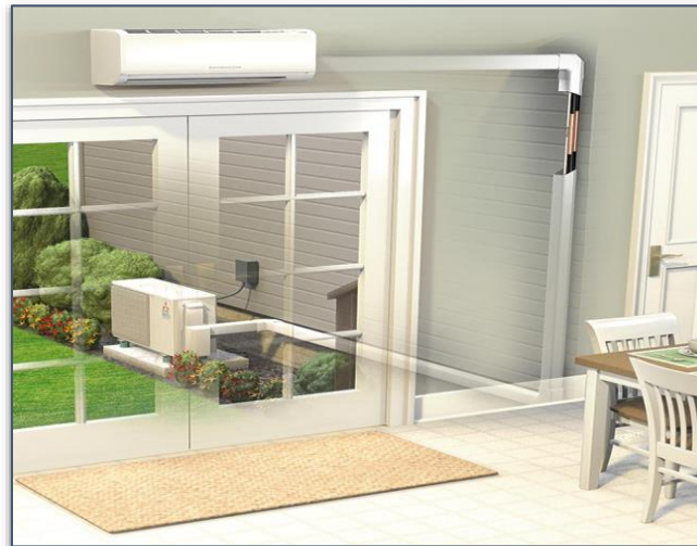
An illustration of a ductless mini-split system.
