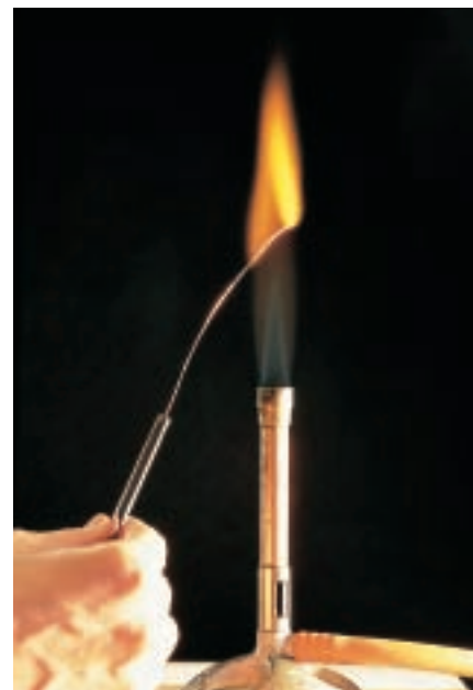
Platinum wire flame test
