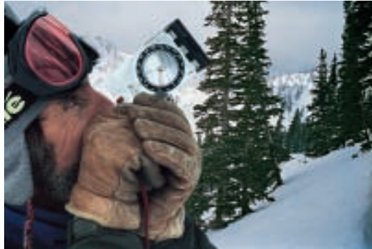
U.S. Forest Service Ranger Al Sousi uses a clinometer to measure the angle of a mountain slope. In snowy conditions, a slope steeper than 35^\circ can be a high avalanche hazard.
