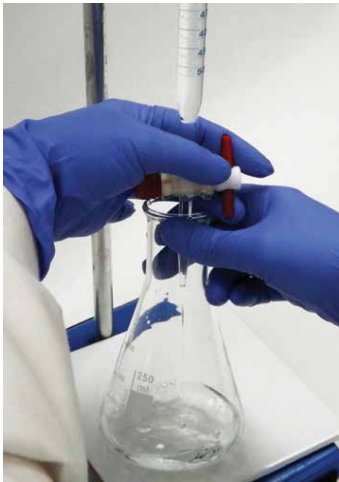
Figure 4 Arrange the tap so that it is on the opposite side of the burette to your palm. That way your hand supports the burette as you operate the tap
