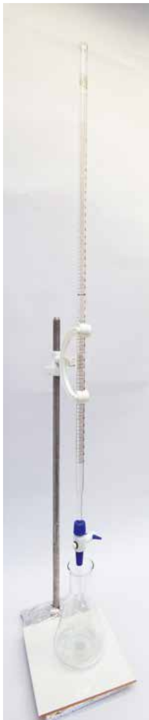
Figure 2 Burette clamp, burette, white tile and clamp/retort stand set up
