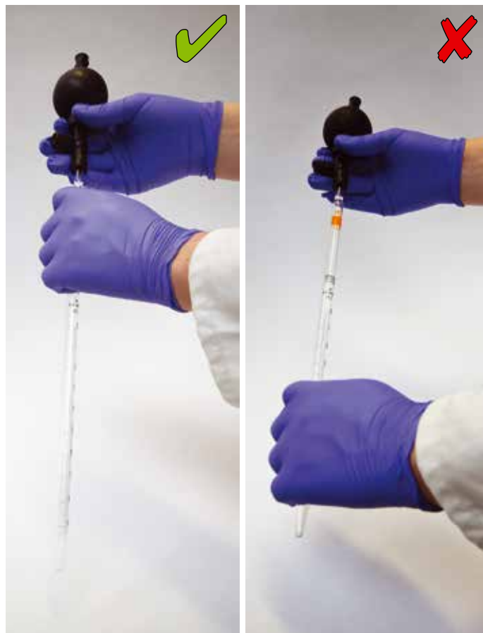
Figure 3 The right and wrong way to put a pipette filler onto a pipette
