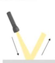
Example: light travelling and reflecting from a rough surface.
