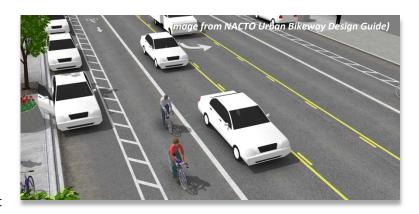
Benefits of buffered bicycle lanes include: providing greater distance between motor vehicles and bicyclists; reduced risk of "dooring"; greater maneuverability outside of the motor vehicle travel lane; and provides for more room for bicycling without creating the perception of an additional travel or parking lane. When properly designed, buffered bicycle lanes encourage bicycling by contributing to the perception of safety among users of the bicycle network.
