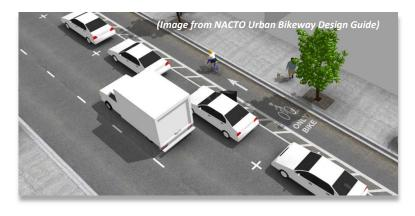
or bollards. By separating cyclists from motor traffic, cycle tracks can offer a higher level of security than bike lanes and are attractive to a wider spectrum of the public.
