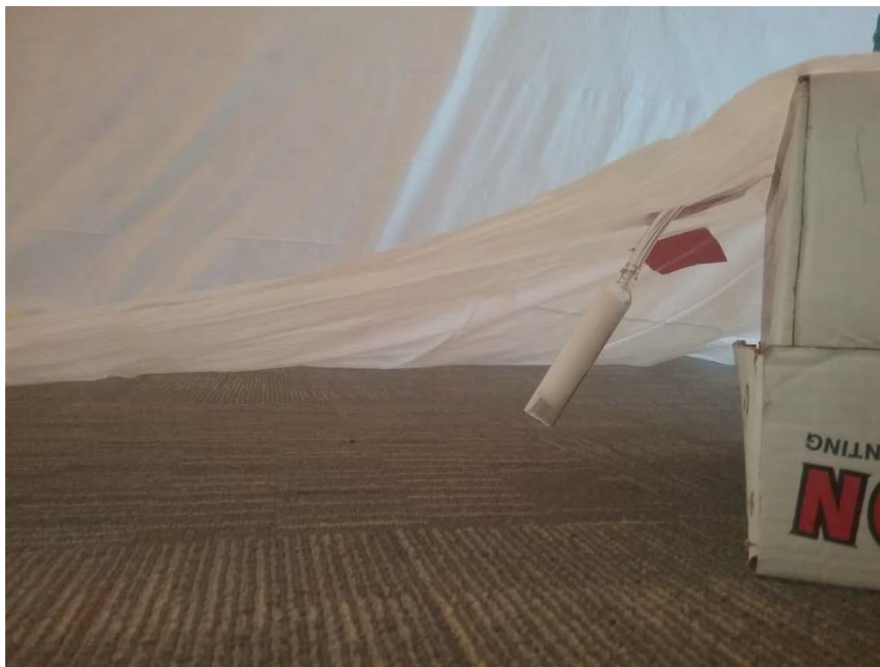
Photo 16 Depicting Side Profile of Floor Sample Apparatus at Carpeted Area. (Barrier cut away following sampling to show configuration)
