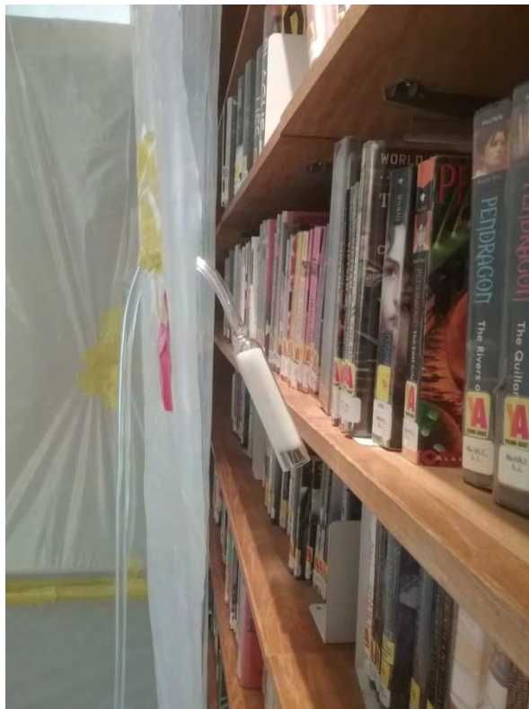
Photo 15 Depicting Side Profile of Wall Sample Apparatus. (Barrier cut away following sampling to show configuration)
