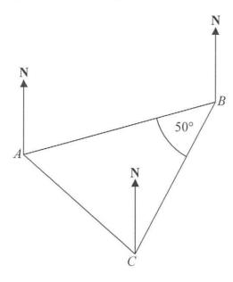
The bearing of B from A is  $070^{\circ}$
