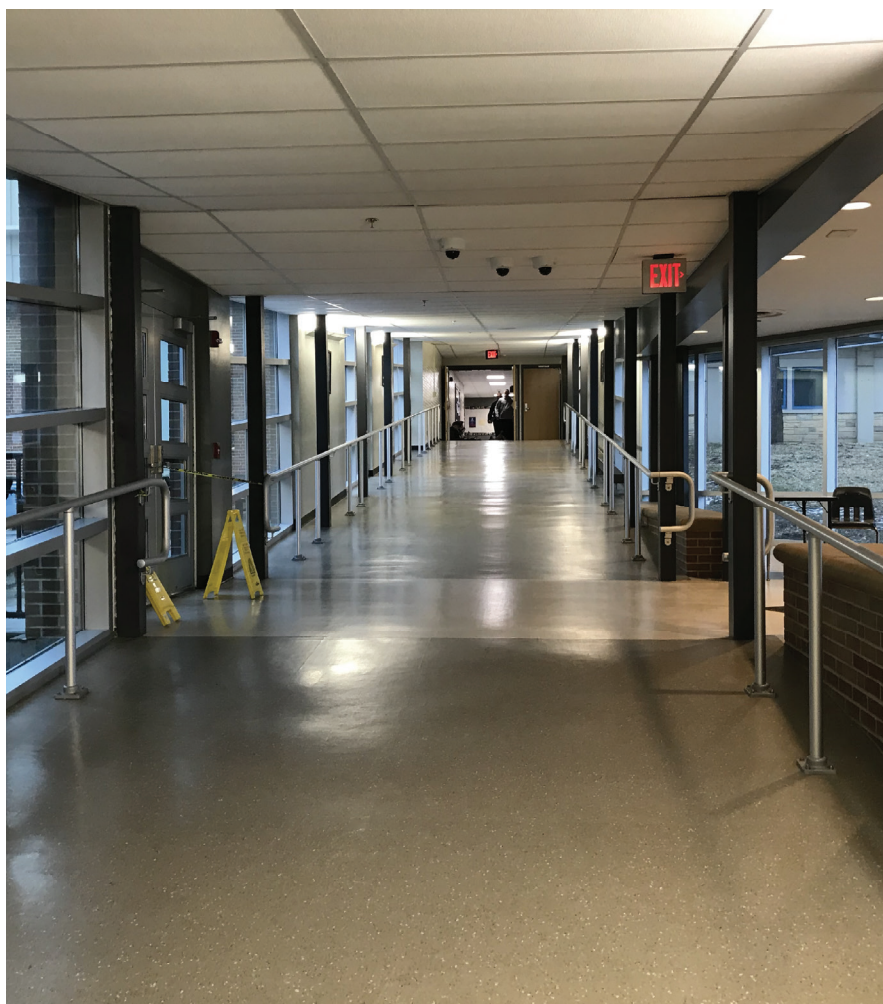
Sloped hallway may not be up to current accessibility standards.
