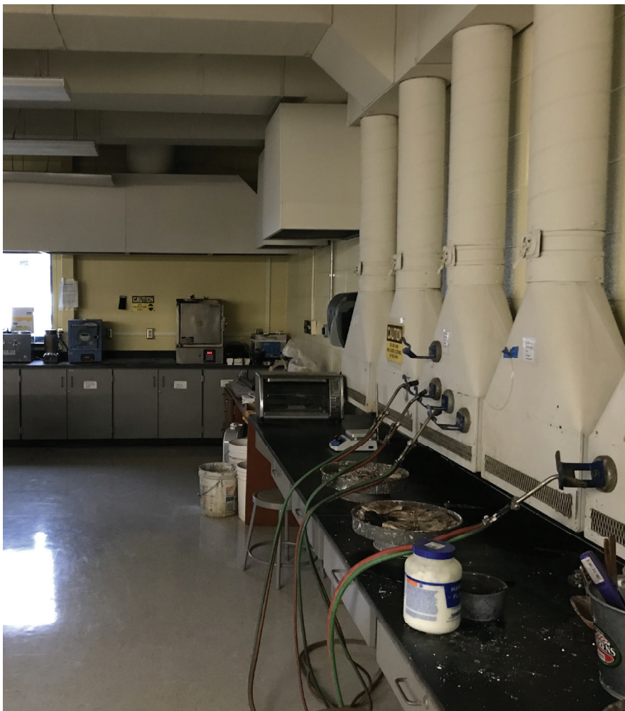
Welding bench is not divided into stations and equipment could use updating.
