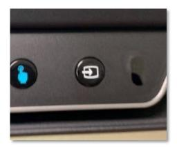
Click **source** button on front of panel. OPS box must be on to appear in sources.
