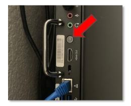
Press **power** on OPS box (located on upper left side of panel).
