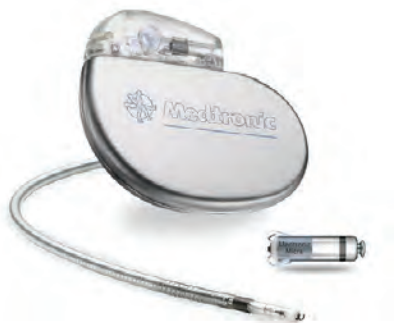
Micra pacemaker (right) compared to traditional pacemaker device
