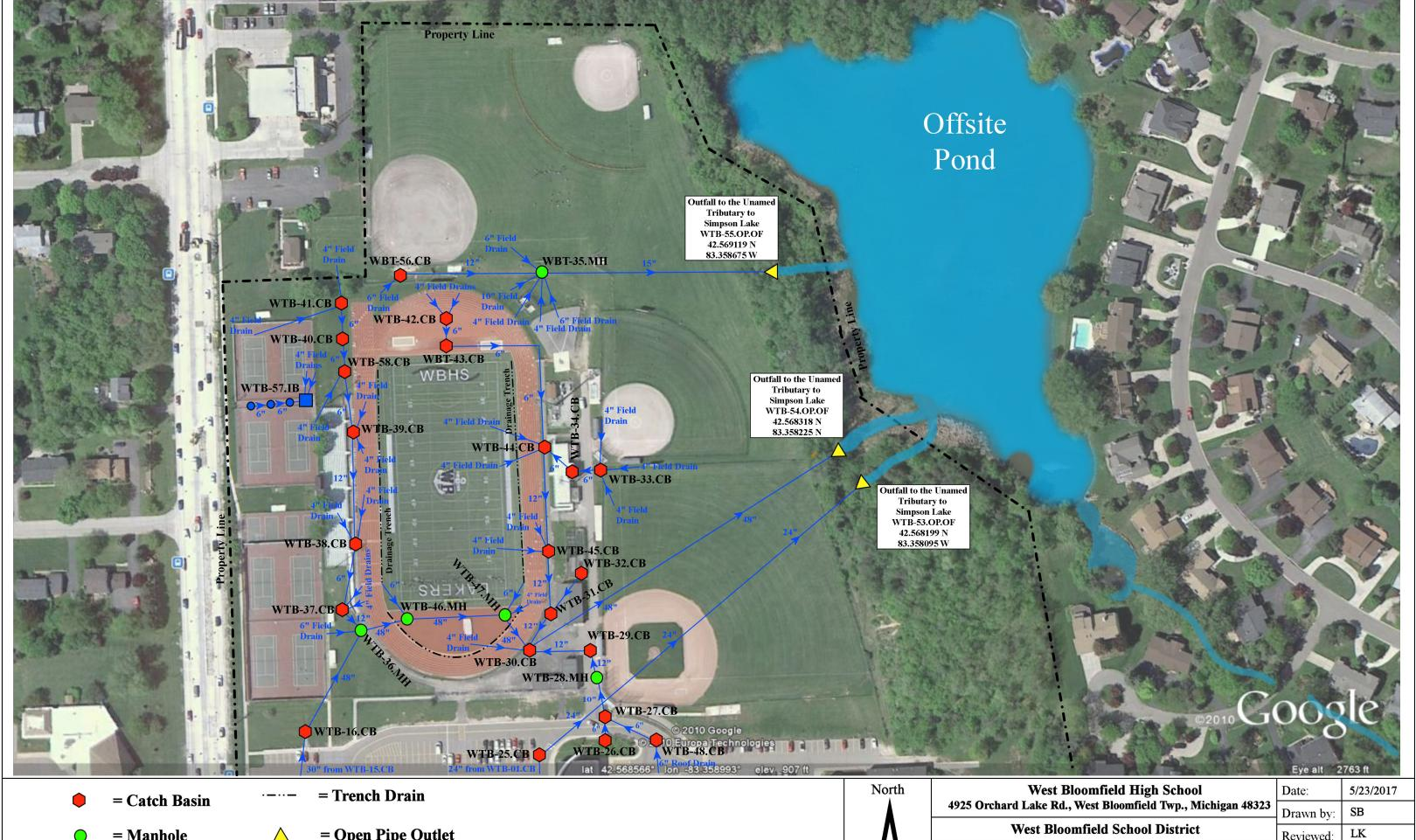
= Manhole = Open Pipe Outlet = Infiltration Basin
