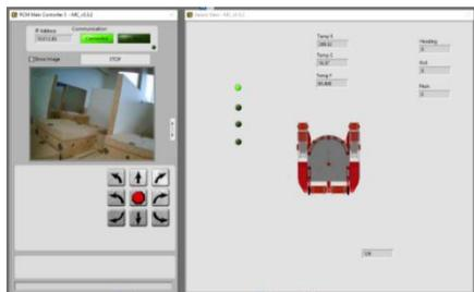
Fig. 11. MainController control interface.
