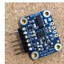
Fig. 6. Adafruit BNO055 9-DOF IMU.
