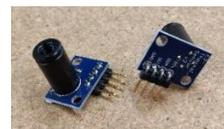
Fig. 7. E3 Thermal sensor with Melexis sensing element.
