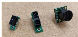
Fig. 5. Sharp digital IR (left), Sharp analog IR (center), Maxbotix Ultrasonic (right).
