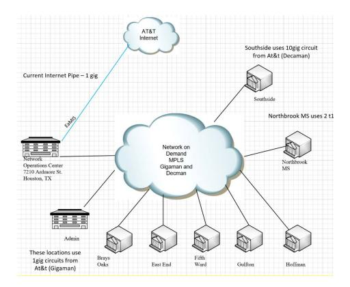
Fiber connectivity between district facilities (this should include pricing options for 10Gbps to each campus) to terminate at Energy Transfer at 7210 Ardmore, Houston, TX 77054. Internet Service must be a managed service with a minimum of 10Gbps.
