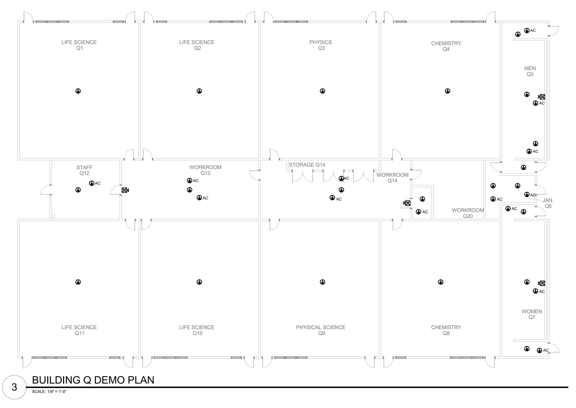
TO REMOVE ALL UNUSED DEVICES, CIRCUITRY AND CONDUIT BACK TO SOURCE.
