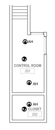
TO REMOVE ALL UNUSED DEVICES, CIRCUITRY AND CONDUIT BACK TO SOURCE.
