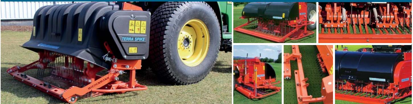
The Terra Spike™ is renowned for speed, precision and easy operation. Welcome the SL at 470 kg our 11th and lightest yet. Specifically for greens and tees, it tines down to 220 mm making it twice the match of any shallow aerator. Pairs with tractors from 20 hp with lifting capacity of 600kg.
