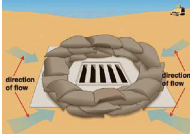
Figure 1. Sand or gravel bags can be used to filter stormwater runoff before entering a catch basin. Commercial products are also available that fit in front of or inside the catch basin.
