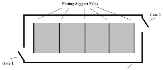
Safety Fence - 6 Gauge Galvanized (2" mesh) Chain Link
